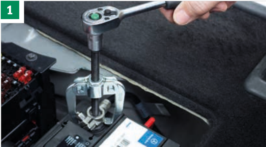
1 Battery terminal puller in use on a car battery
