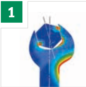
Load zones in standard-quality spanners
