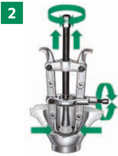
2 How a two-armed puller works
